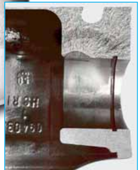
Fig. 2 cross section of the piston pin boss
